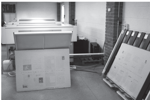
Figure 2. Journal pages etched on aluminium printing plates.
